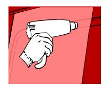
8. Now, start stretching the material in the corrugation, starting in the deepest part of the corrugation first. Make sure that the material is heated to remain at the 105°-125°F (40°-50°C) temperature.
