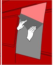
When edges and corners are resqueegeed, make sure the material is fixed on the edges of the corrugation (see below), and work your way around the entire corrugation, just fixing the edges.
