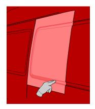
12. Check the application for remaining bubbles. If there still are small air bubbles to be seen, these can easily be removed. Just make a small puncture, heat it a little and push the air out.
