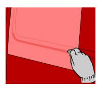
10. When all the deepest parts of the corrugation have been applied, the inside of the corrugation can be done. Again, make sure the material is heated to the required 105°-125°F (40°-50°C), and work you way through the corrugation.
