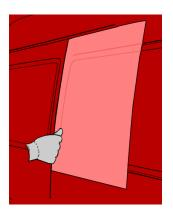
Now the application of the material in the corrugation can start. In order to be able to do so without forming wrinkles or creases, it is advised to wet the glove, using a water/soap mixture.
