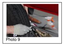
• Keep the squeegee edge wet during the entire application process, paying attention to rewet the squeegee upon final re-squeegeeing of all edges, and the entire graphic to ensure secure adhesion to the substrate. As shown in photo 10.
