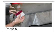
• Work the film gently around edges and curves using a wet edge squeegee, wet application glove, and light heat as shown in Photos 6, 7, 8
