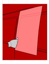
Now, the application of the material in the corrugation can start. In order to be able to do so without forming pleats or creases, it is advised to wet the glove, using a water/soap mixture.
