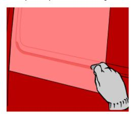
When all the deepest parts of the corrugation have been applied, the inside of the corrugation can be done. Again, make sure the material is heated to the required 40°-50°C, and work you way through the corrugation.
