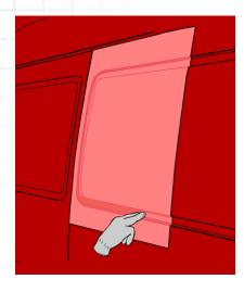
Check the application for remaining bubbles. If you see any small air bubbles, remove them by making a small puncture, heat it a little and push out the air.
