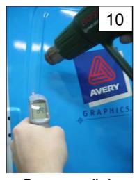
Remove small air bubbles first (if present), and then reheat the stretched areas until 80-90°C.
